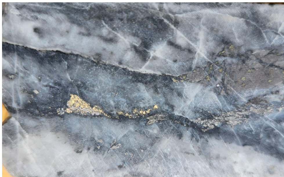
Figure 1: Intersection in Upper Crown DDH24-093 – NQ core 161.3 m - Visible Gold in Quartz Vein
